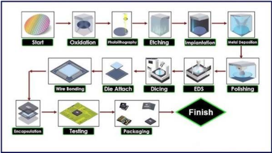
Fig. 4: Semiconductor manufacturing process flow chart
